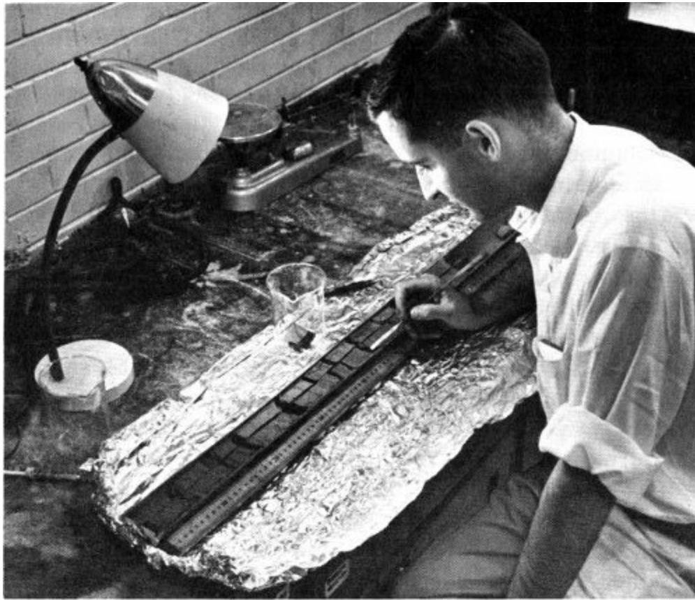
Examining ocean-bottom sediments obtained by lowering a tube-like instrument that brings up a long rod-shaped “core”, prior to nuclear age determination of the sample.
